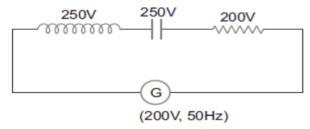
Algebric sum of voltages =  $V_R + V_L + V_C = 200V + 250V + 250V = 700V$
